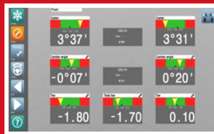
Live simultaneous readings of castor, camber and toe
