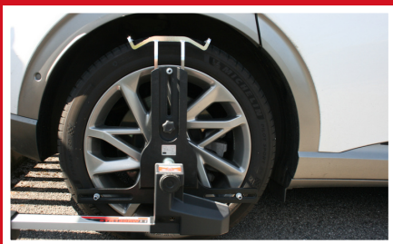
Effective hang on system for full 4 wheel alignment measurements
