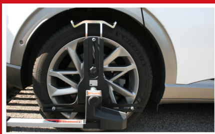
8 sensors allows measurement of rear set back
